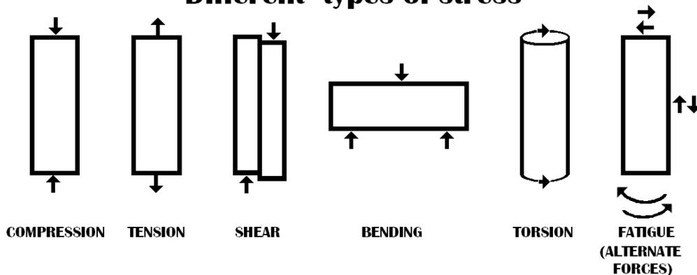
Figure 9. Different stress types which can be caused by an earthquake on a building. (Almazi, 2016)
