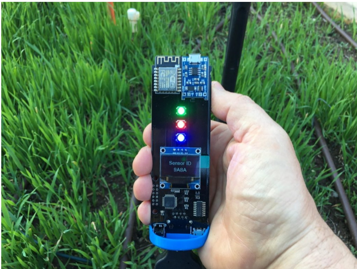
CSIRO's chameleon device - a simple hand-held sensor which allows water and nutrients levels to be measured.
