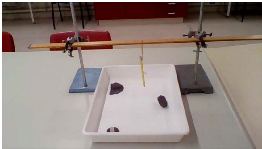
Figure 8. Set up with magnets/ magnetic minerals in tray (this should be covered in sand). Magnet on hook is suspended above by an elastic band and should be attracted to the hidden magnetic items as it passes over them.
