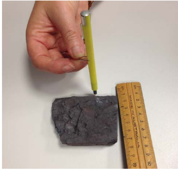
Figure 4. Testing the magnetic strength of different samples - measuring how far away the magnet is attracted to the sample.
