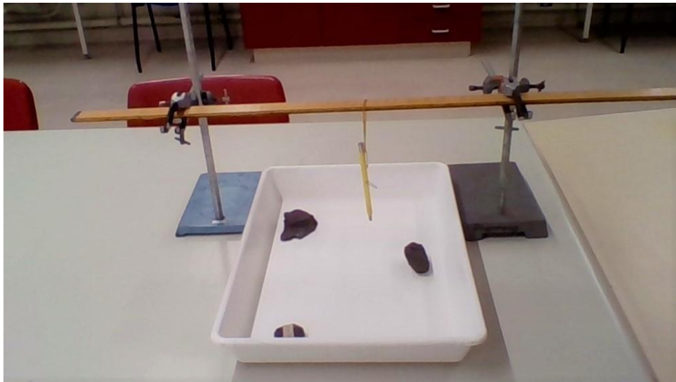
Figure 9. Set up with magnets/ magnetic minerals in tray (this should be covered in sand). Magnet on hook is suspended above by an elastic band and should be attracted to the hidden magnetic items as it passes over them.
