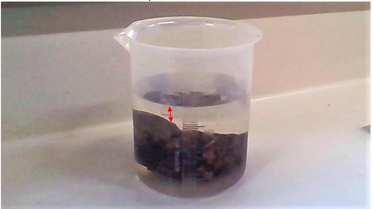
Figure 5. If you have a smaller sample you can measure the difference in the level of water before and after a rock is placed into the beaker.
