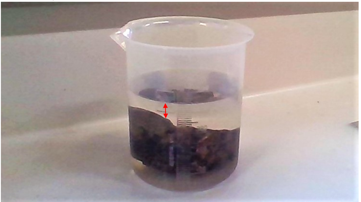
Figure 4. If you have a smaller sample you can measure the difference in the level of water before and after a rock is placed into the beaker.
