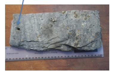
This rock is a roof slate. During metamorphosis pressure changed and aligned its minerals making it waterproof and able to be split into flat plates. Some of the dark marks on its surface are from fire smoke. The hole at the end was to allow it to be nailed to wooden roof beams.
