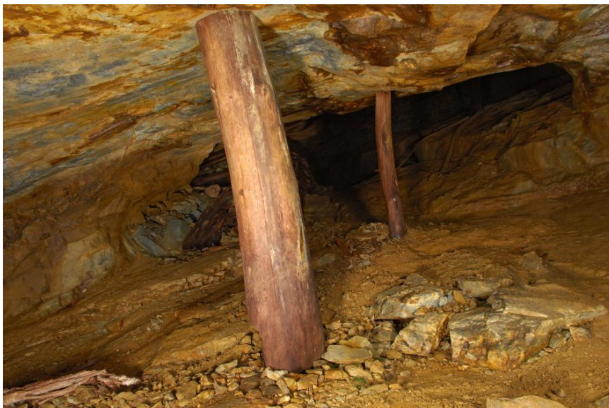
Pit props used to support the roof of an old stope in Hannans gold mine in Kalgoorlie.
