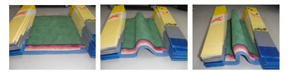
This activity demonstrates the formation of anticlines (domes) well but does not demonstrate synclines (down warp) as the table surface restricts downward movement. Continental crust however can down warp into the underlying denser oceanic crust. Most large mountain ranges such as the Himalayas have deep 'roots". These mountains are being forced upwards by the northward movement of the continent of India.
