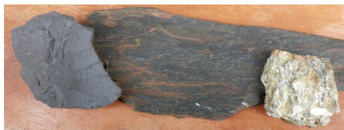
Progression from mudstone on left, to slate in centre to schist on right
