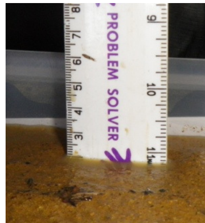
Height of sand + water 2.5cm or less
