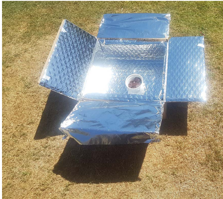
Figure 3. Chocolate melting in a solar oven with four flaps
