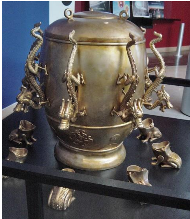
Figure 3. The ball would be released from the mouth of the dragon in to the frog's mouth to indicate which direction the seismic wave was moving.
