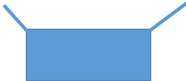
Figure 3. Solar oven with two flaps angles at ~ 45 degrees
