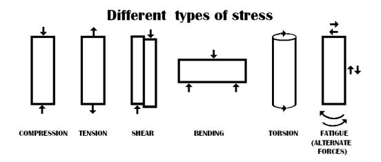
*Figure 9. Different stress types which can be caused by an earthquake on a building. (Almazi, 2016)*
