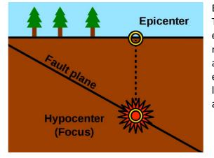
Figure 2. Diagram of the epicenter of an earthquake, where movement along a fault plane has caused it. (Hocevar, 2014)
